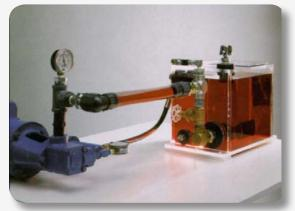
Participants see first-hand how problems such as cavitation, aeration, erratic pressure, loss of pressure or flow shorten component life and influence system failures.
