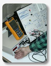
Participants verify the function of both a three-way and four-way switch by using a DMM to test each switch. Additionally, participants will determine how to connect wires to the terminals for a complete electrical circuit that can be operated from multiple locations.
