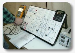
Participants will measure resistance and AC voltages in a series of circuits and parallel circuits.
