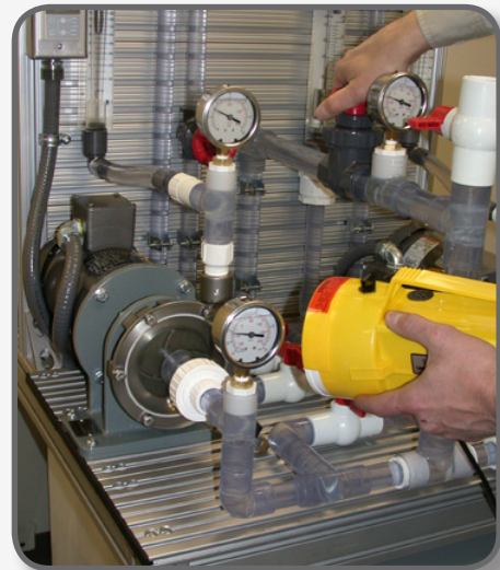
Using a strobe light on the NTT training equipment to demonstrate cavitation.
