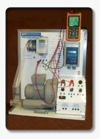
The advantage of using Variable Frequency Drives (VFDs) is their energy saving potential. Students calculate the enormous energy savings using data from live measurements, and plot the data to show the energy savings VFDs offer over standard HVAC speed control designs.
